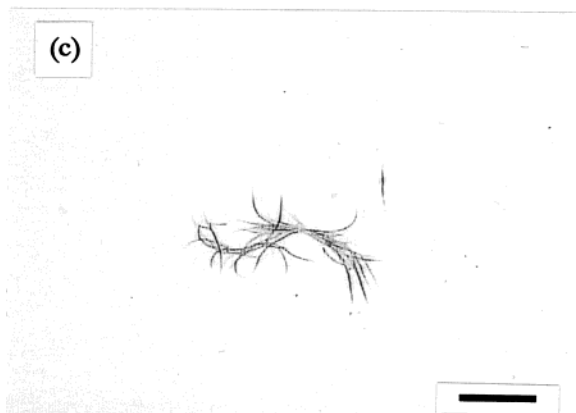
Figure 7. Optical microscopy images of molecular assemblages formed from 4b (a) in the dark, (b) under irradiation with light at >350 nm, and (c) with UV light at 365 nm, respectively (scale bar: 100 \mu m).
